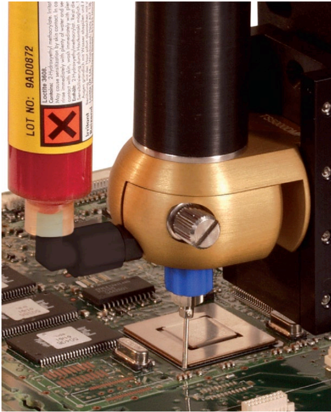
TS5000DMP - Performing underfill
